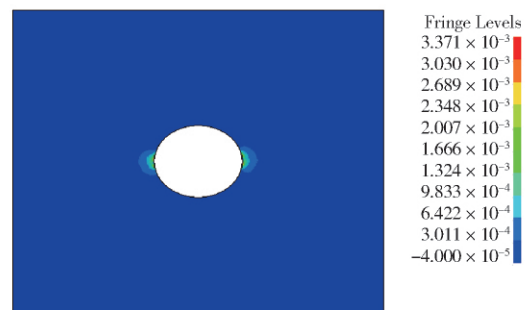
(c) t = 11.4990 \times 10^{-6} s 时的应力云图
